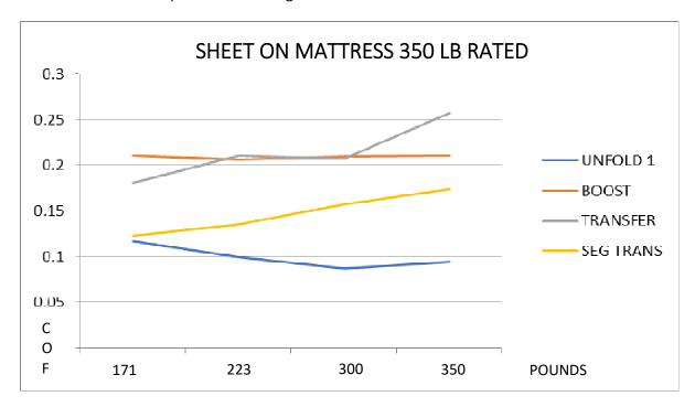
The kinetic COF lines in the above charts used the "Max" data from the following chart "FORCE REQUIRED TO MOVE PATIENT ON DIFFERENT SURFACES USING PATRAN SLIDE SHEETS." Use "Min" data to calculate the static COF.
